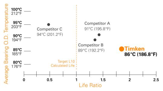
Tested 22212 at 2700 rpm with a load  $^{\sim}25\%$  of the dynamic capacity.
